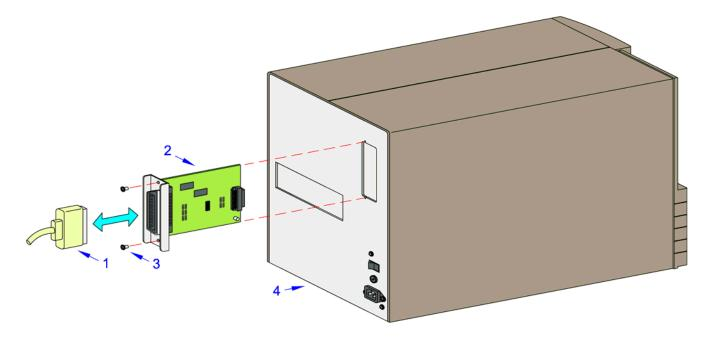
Figure 6-2, Interface Board Replacement
